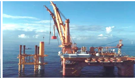
SEMI Conversion to WTIV Delivered: 2021 Capacity: Huisman 1800t *2 Working in South China Sea
